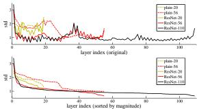
Figure 7. Standard deviations (std) of layer responses on CIFAR-10. The responses are the outputs of each  $3 \times 3$  layer, after BN and before nonlinearity. **Top**: the layers are shown in their original order. **Bottom**: the responses are ranked in descending order.
