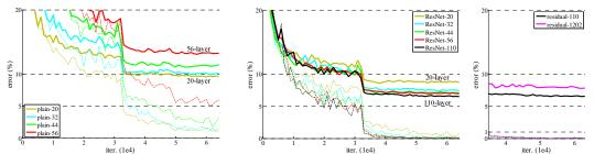
Figure 6. Training on **CIFAR-10**. Dashed lines denote training error, and bold lines denote testing error. **Left**: plain networks. The error of plain-110 is higher than 60% and not displayed. **Middle**: ResNets. **Right**: ResNets with 110 and 1202 layers.
